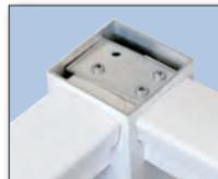
Predrilled rail tabs are provided with the post to connect the top rails. If a railing section or sections need to be shortened, simply saw an equal amount from each railing end with the use of a miter or circular saw. Reinstall and tighten the rail wedge using an 1/8" Allen Wrench on the bottom rail so 1 1/4" protrudes through the post openings. Next, connect the two top rails together with a rail tab, and drive the post cap in place with a rubber mallet.
